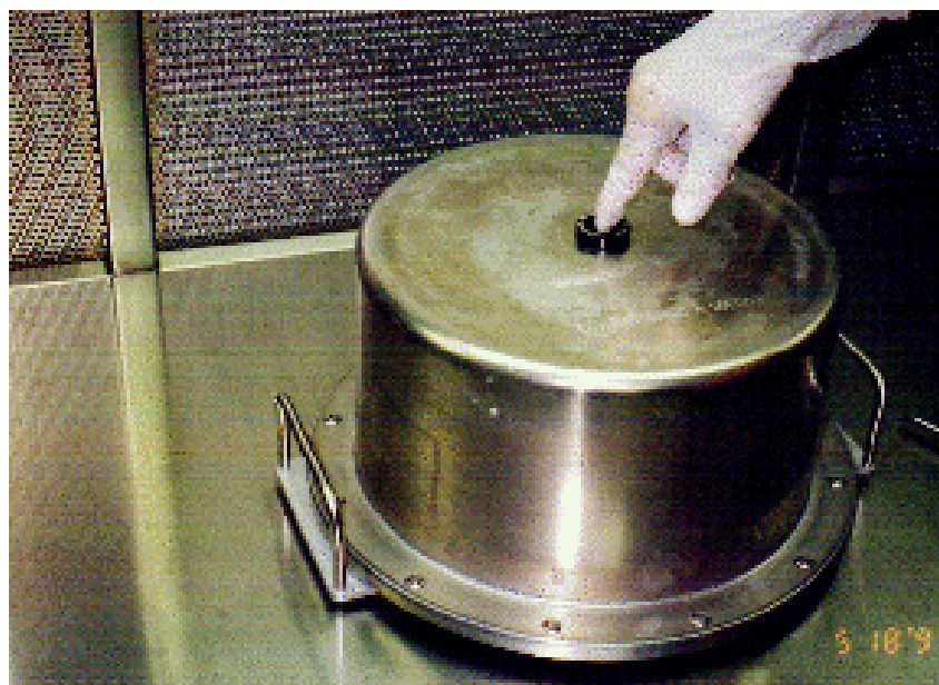
Figure 5, Note: The pressure/vacuum release valve shown being manually depressed has been excluded as of revision C of both carrier designs.
