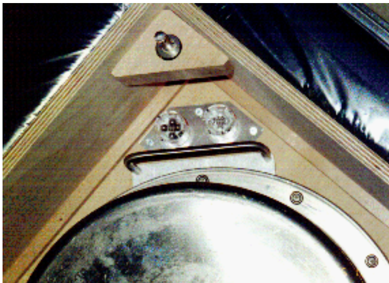
Figure 4: 60g & 150g Shock Indicators
