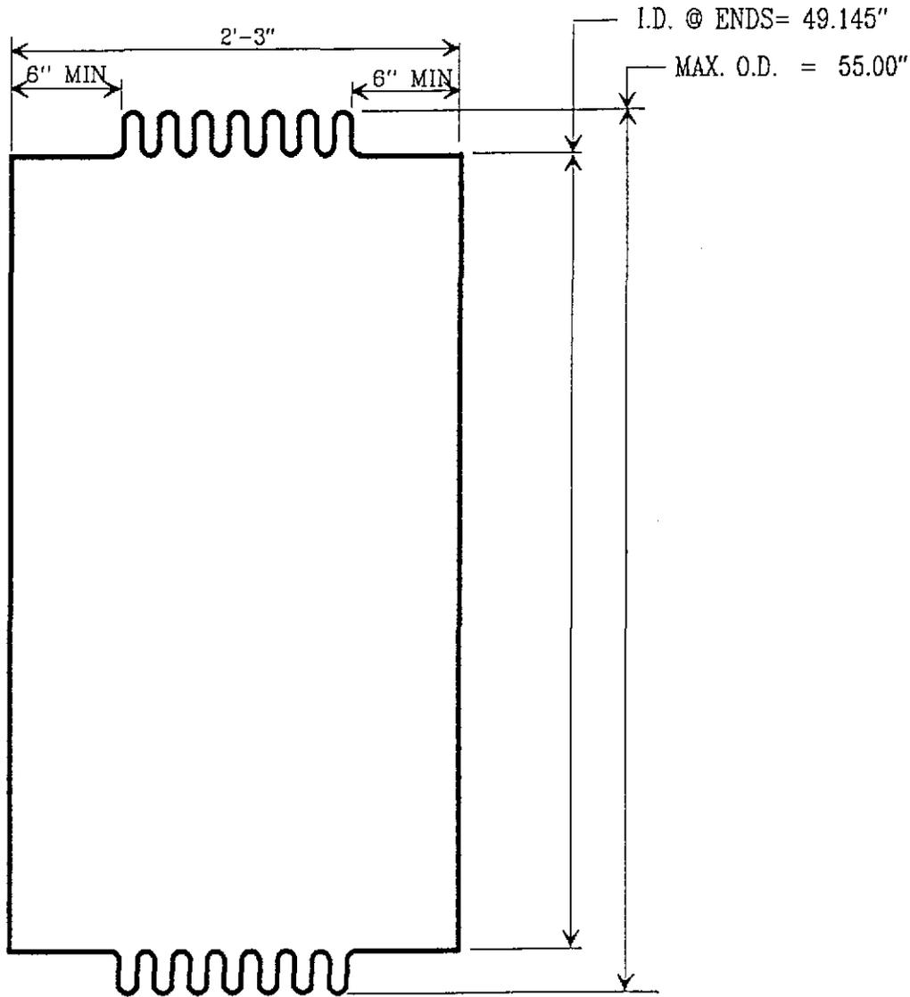
FIGURE 2 - EXPANSION JOINT DIMNSIONAL LIMITATIONS
