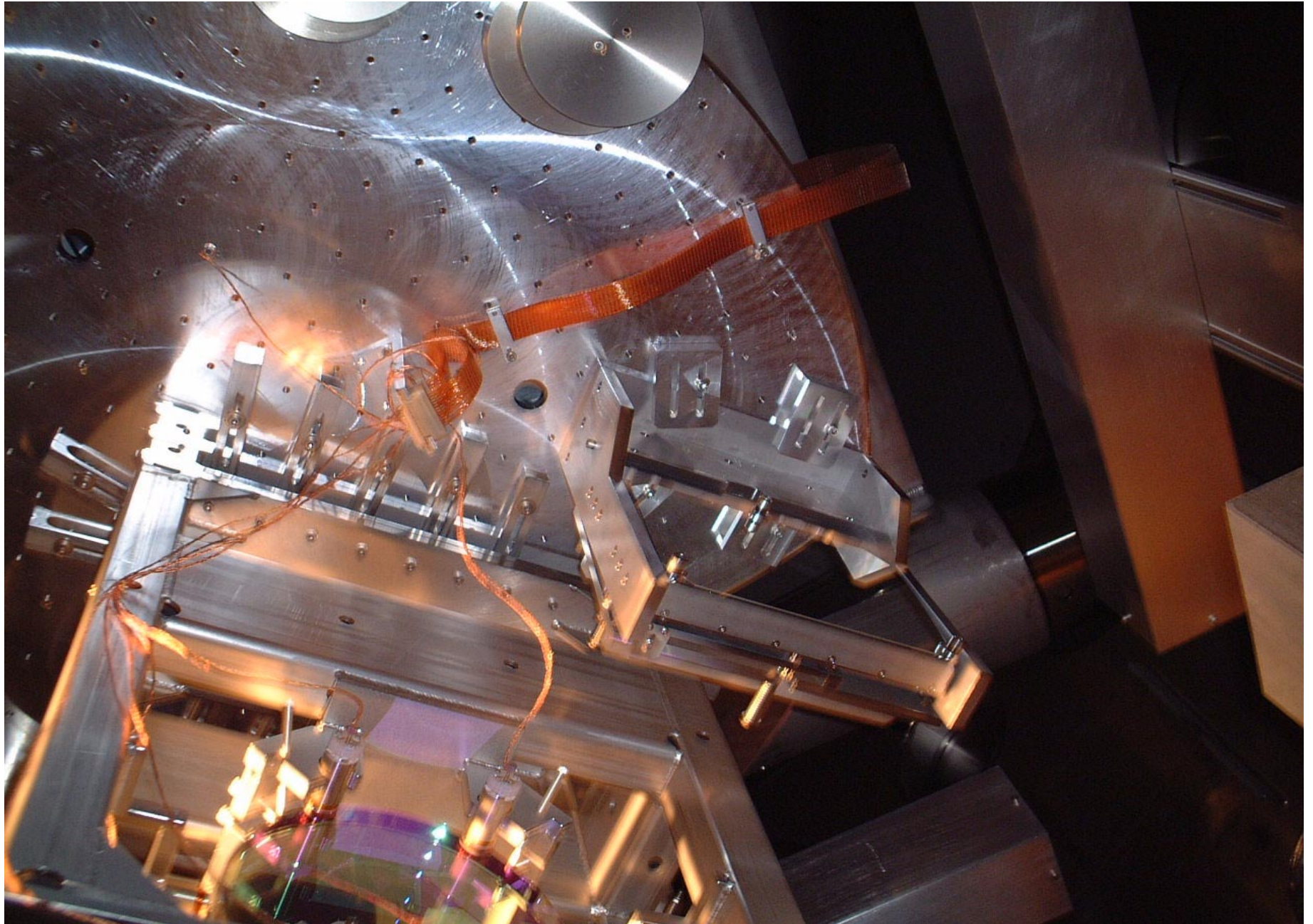
BSC4 BS AR surface as viewed from below optics table. ITMy Pick Off mirror is in the center of the picture. COS beamdump tube hangs at the top of the South entrance to the chamber at the far right of the picture.
