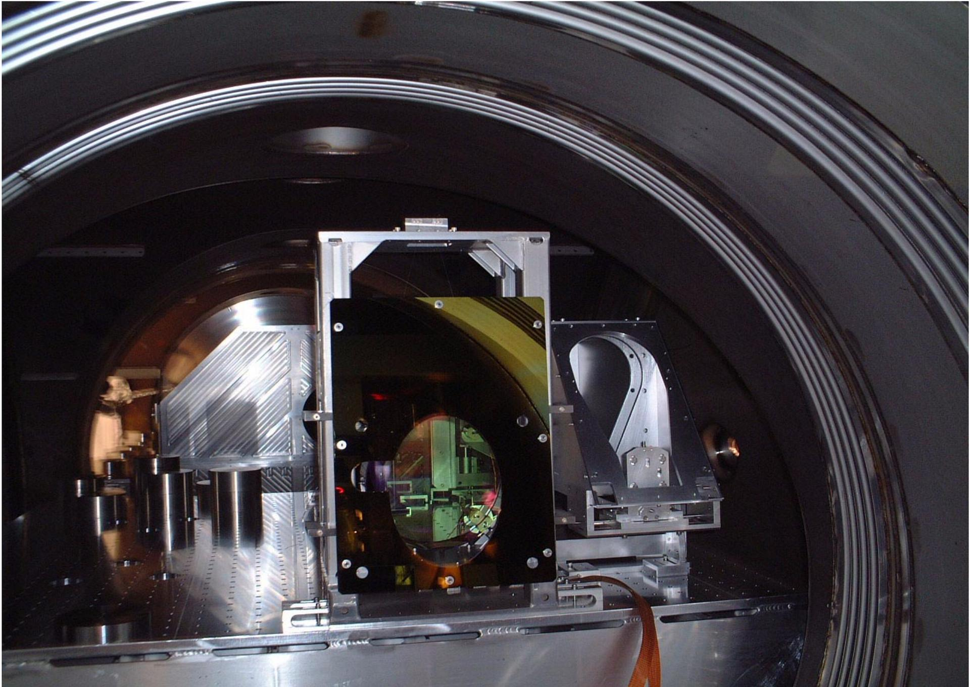
HAM9 Looking North at the Recycling Mirror (RM), elliptical baffle, IO baffle (background), and ITMx PO Telescope (right).
