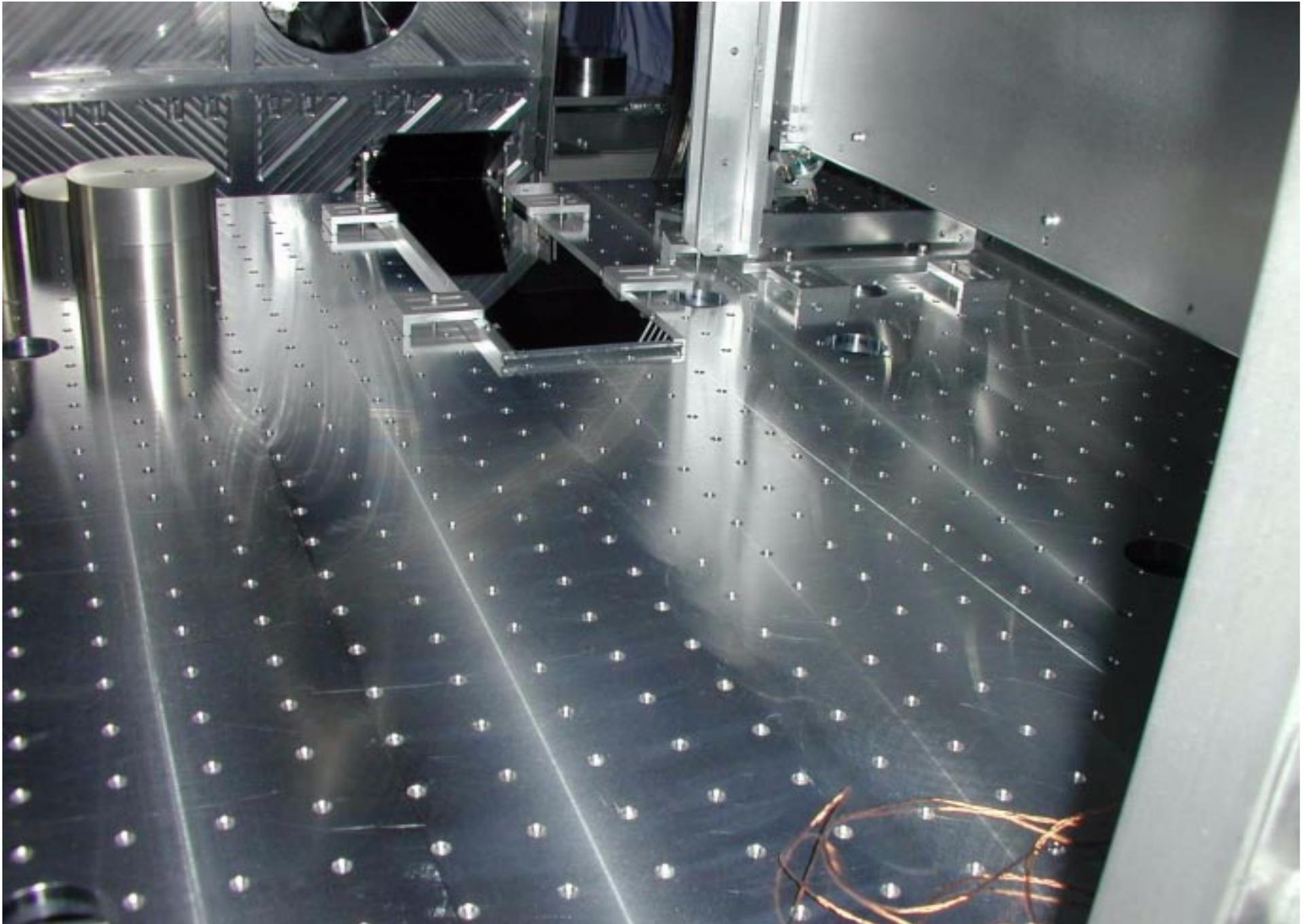
HAM( COS Beam Dump at North edge of table. IO baffle is at the top, PO Telescope is on the right.
