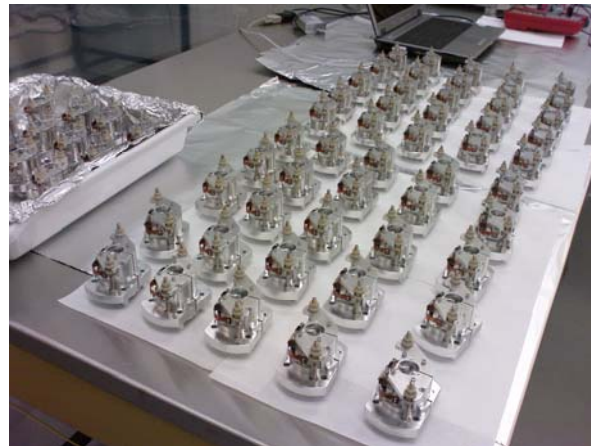
Assembled BOSEMs at ATE station
