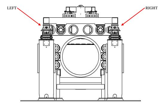
2. If positioned on a correctly identified LEFT side pier, create a punch mark through the two ½" clearance holes labeled LEFT (hole locations as shown below).
