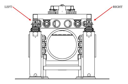
2. If positioned on a correctly identified RIGHT side pier, create a punch mark through the two ½" clearance holes labeled RIGHT (hole locations as shown below).
