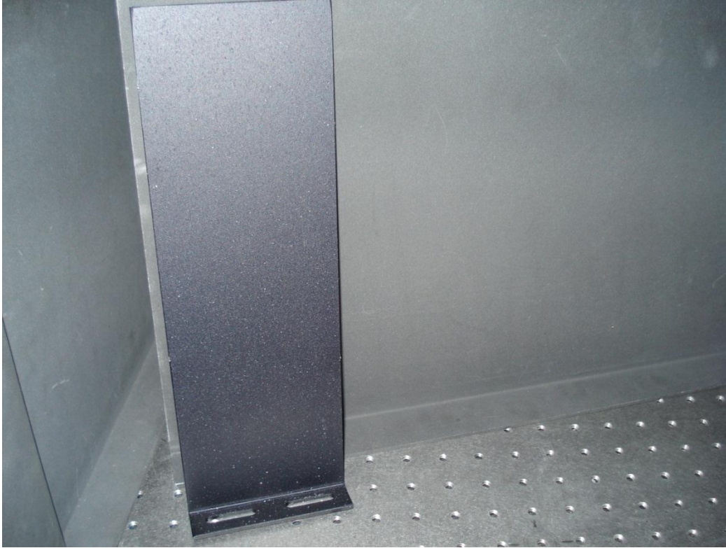
Figure 7: A plate style beam dump.
