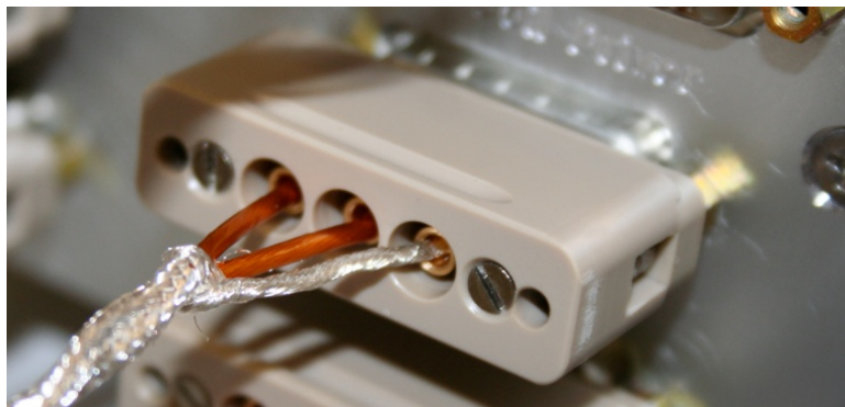
Figure – Actuator cable plugged on the feedthrough
