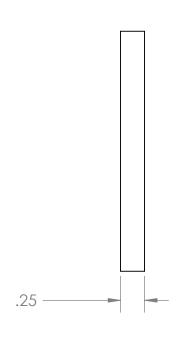
DESCRIPTION: PLATE, .25 THK, 2.50 WD, 4.00 LG MATERIAL: AISI 304/AISI 304L DUAL CERT PER SA240 UNLESS OTHERWISE SPECIFIED: WEIGHT: 0.62 # DIMENSIONS ARE IN INCHES
