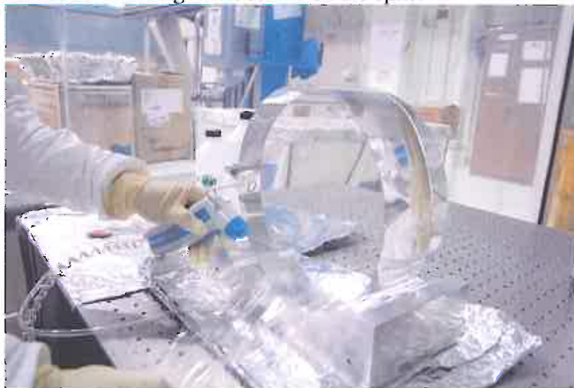
Figure 5: Keep a steady stream of nitrogen while peeling.
