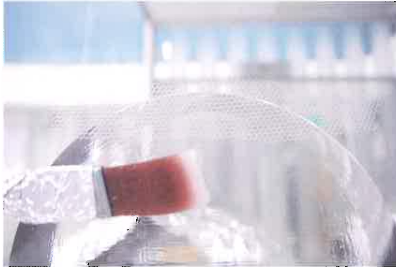
Figure 4: Leave mesh sticking up enough to grab it for removal. Note: The mesh in this picture is nylon mesh, not PEEK.
