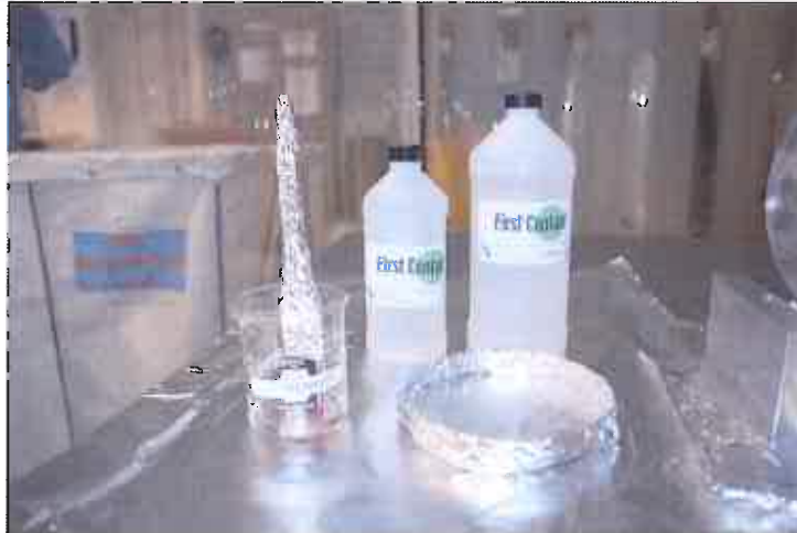
Figure 1: To keep from having sticky petri dishes, wrap them in foil, pour in the FC and then discard the foil when finished.
