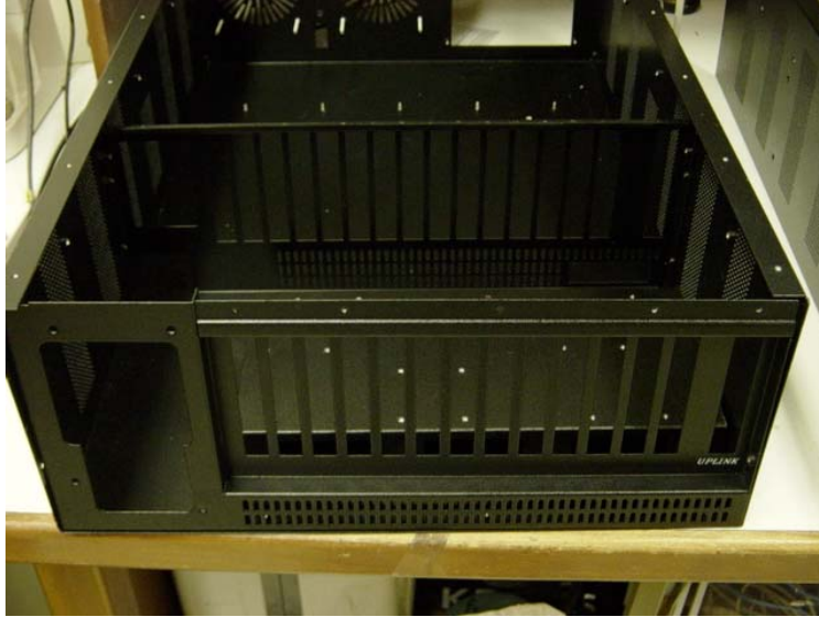
Figure 2: Chassis Base with Rear Panel and Internal Bracket, Internal Panel and Rear Bottom Panel Installed
