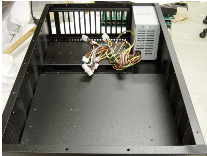
Figure 3: Power Supply Mounted in Chassis Base. Note that Internal Panel has been removed for picture and the power supply being installed may be slightly different than the one shown.
