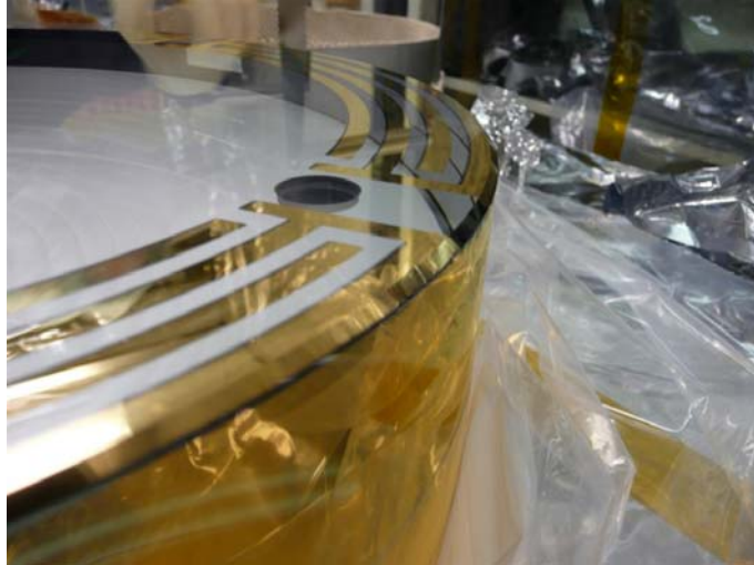
Figure 5.2 Electrostatic drive coating over the chamfer, 1 mm away from the barrel coating
