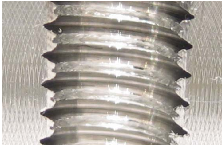
Figure 3: Section through Tap #13 in aluminum, showing “W” form of thread crests caused by thread forming tap.
