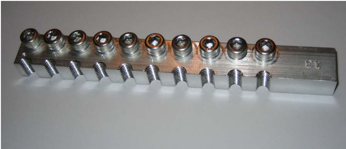
Figure 1: Typical tap block; odd-numbered tap sequence holes (sectioned, for examination) are across the bottom, from left to right, 1 through 19. Even-numbered tapped holes are across the top, 2 through 20. Only the even-numbered holes were tested.
