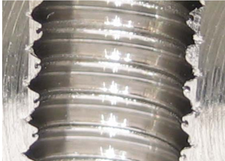
Figure 6: Section through Tap #13 in stainless steel, showing rolled-over “W” form of thread crests caused by thread forming tap.
