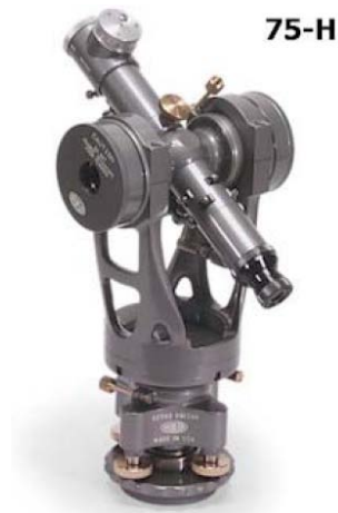
Figure 6 Brunson Optical Transit Square (model 75-H)
