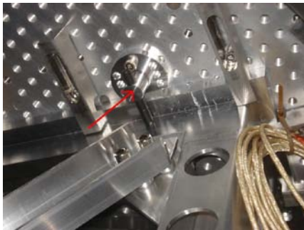
Figure 27 Pusher used to adjust the quad suspension position at LASTI
