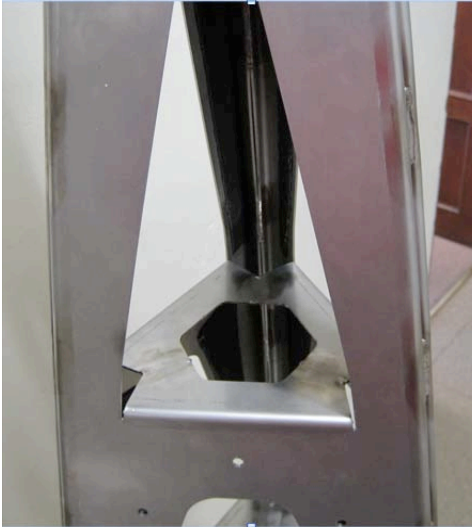
Figure 6. Detail of pylon's folding and welding structure, the folded lips of all windows are welded together for added stiffness. The edges of the three separate panels are folded at 30° angle, then stitch welded forming three very strong ribs along the pyramid sides. Note the black vibration damping adhesive tape near the folded ribs that damps resonances on all surfaces.
