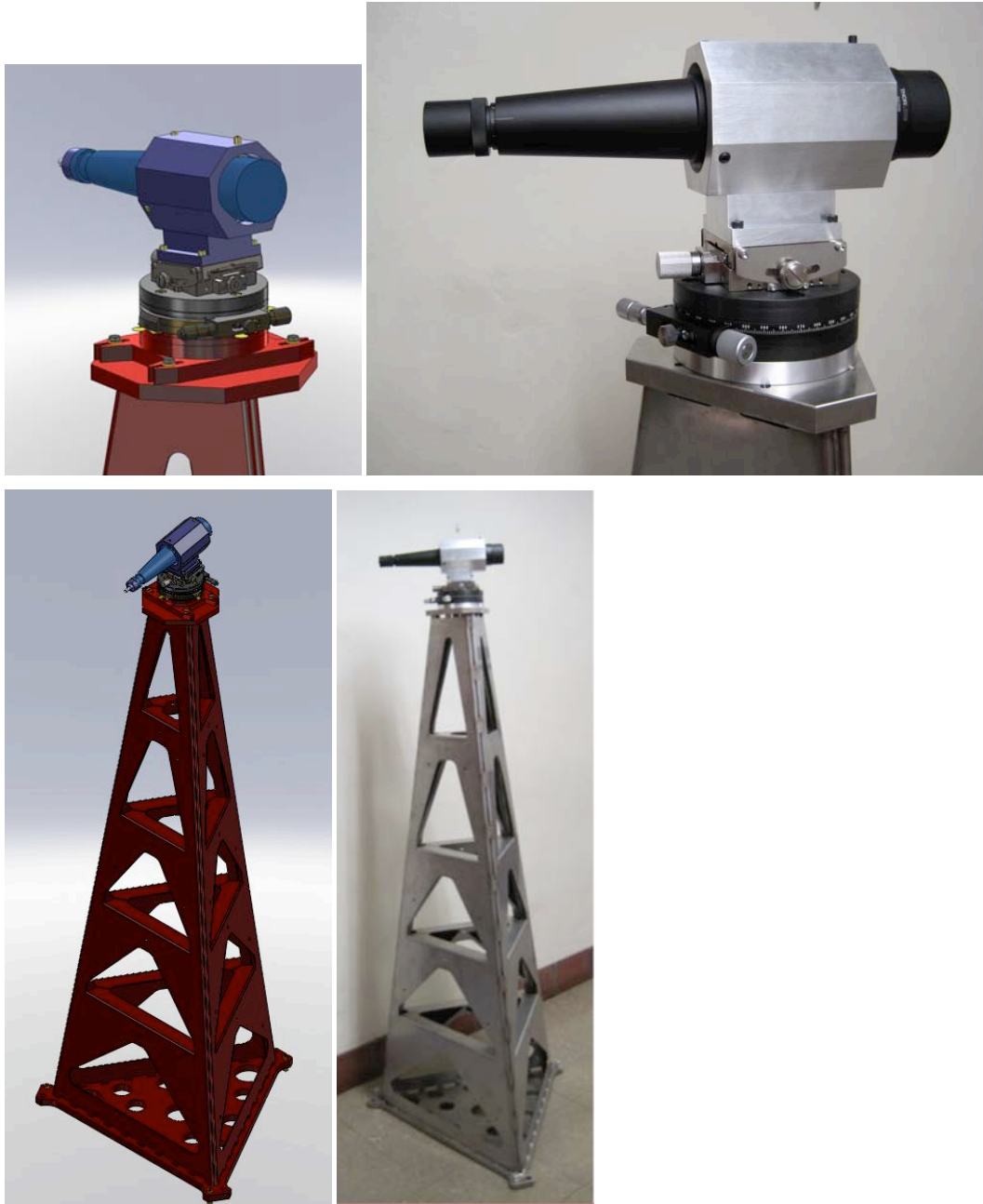
Figure 5. Schematic design of a light pylon to carry the optical lever launching and receiving optics and of a launching telescope to be mounted on top of the pylon. The pylon is made with sheet metal laser cut, bent and stitch welded. The thicker base plate would be bolted to a second plate grouted to ground for maximal stiffness; the grouted plate is provided with large holes to allow the grout to mushroom through, expand and lock the structure to ground.
