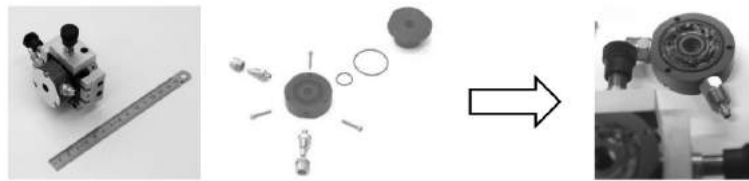
Figure 11.1: Effect of standing water in the water cooled fiber bundle mount. Left: new part, right: effected part.
