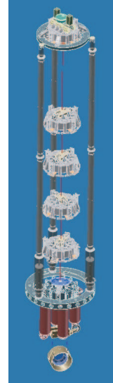
Fig. 4. Superattenuator to be used in Advanced Virgo and LCGT. The three tall grey bars on the outside are the inverted pendulum. Below the top of the inverted pendulum a round stage is supported that contains the blade springs with the geometric anti-springs. There are multiples stages of pendulums supporting blade spring wheels. At the bottom is a control platform that supports the test mass.
