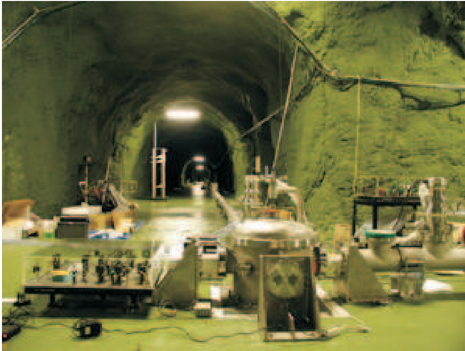
Fig. 5. Photograph of CLIO equipment underground at the Kamioka mine in Japan. Shown are vacuum tubes and input optics for the interferometer.
