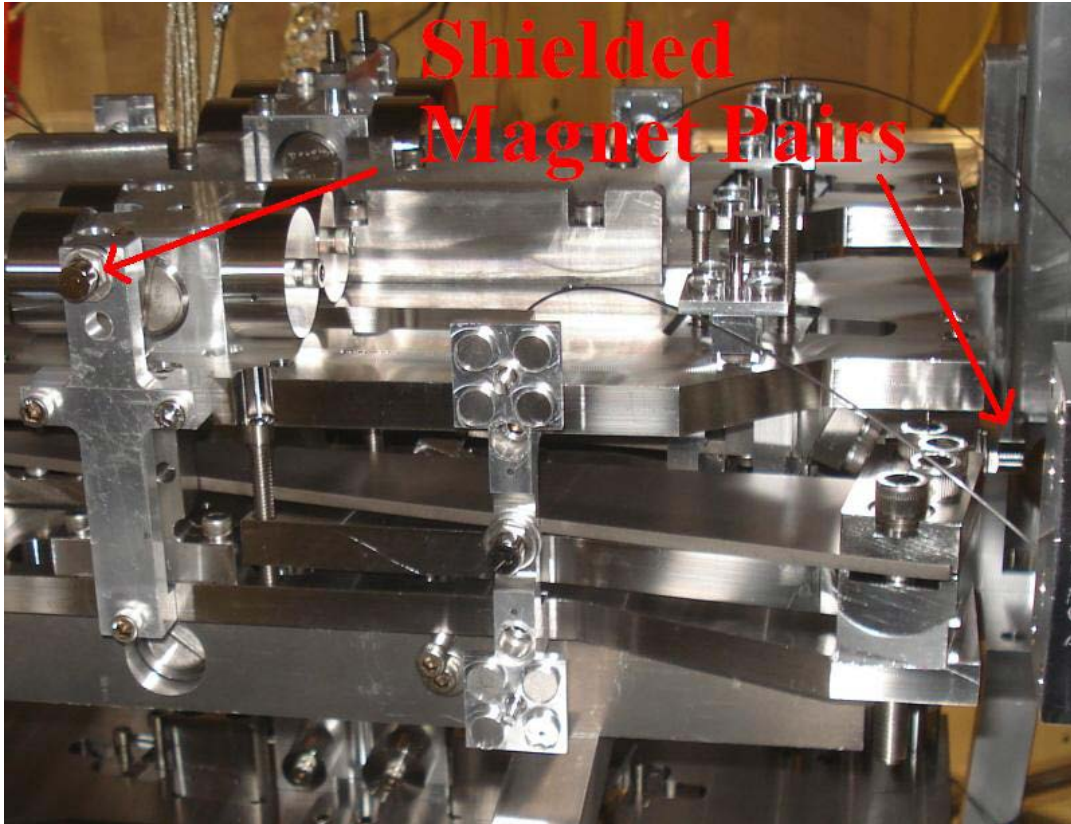
Figure 13 This photograph shows the locations of the shielded magnet pairs around the top mass. In LASTI notation these are the magnets belonging to the 'Side' and 'Face 1' OSEMs. The UI mass OSEMs also have shielded magnet pairs.
