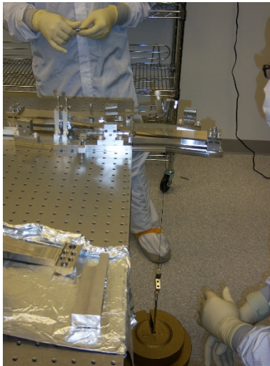
Figure 7 UI Mass with hanging weight to pull blade flat
