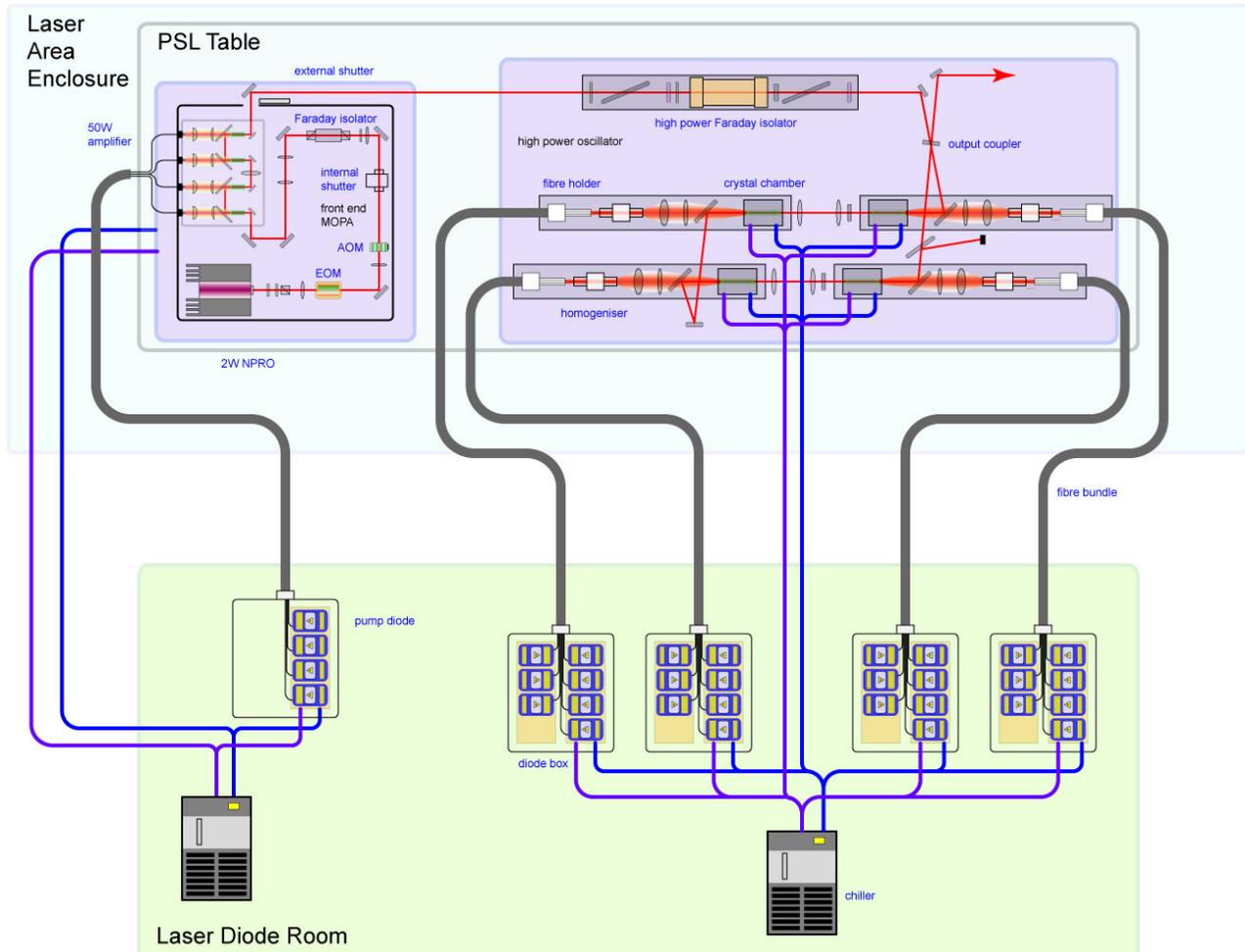
**Figure 1.** The major components of the Advanced LIGO Laser.
