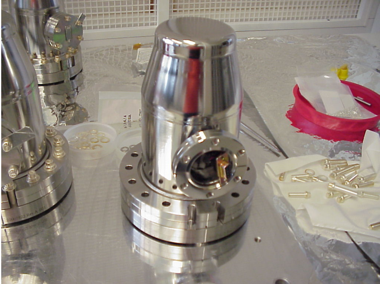
Figure 7: L4-C Pod Chamber Top Hat (D047823) over the L4-C Pod Base Plate (part D047822), with the vertical edge lines aligned on both part
