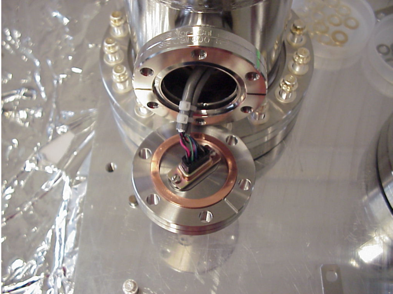
Figure 9: Cable installed onto Flange Feed Through with 2.75" CF Gasket. Ready for Neon Fill
