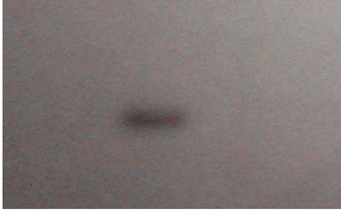
FIG. 24: Visible damage on SiC with 200 \mu\text{m} spot size and 80 W power.
