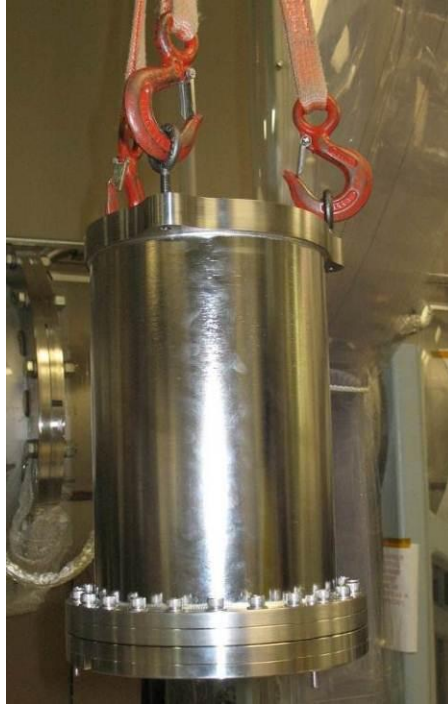
Figure 136: Vertical GS-13 being craned over the Assembly
