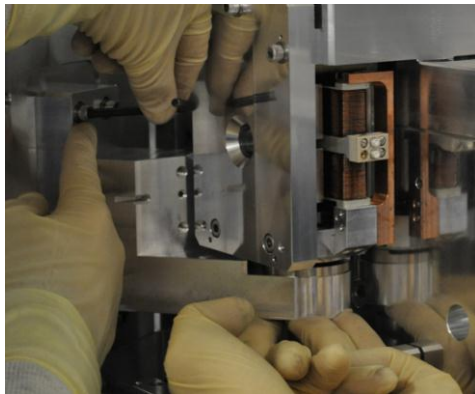
Figure 146: D0902236 Stage 1-2 Actuator Vertical Bracket is flush against D0902278 Stage 1 L4C Wall before tightening the 1/2"-13 x 2.5" HHCS Bolt
