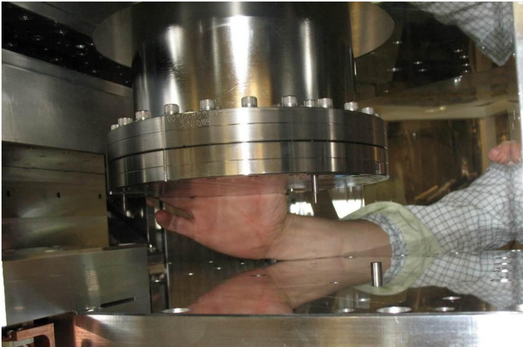
Figure 138: Lowering a Vertical GS-13 in place (LASTI dirty Assembly)
