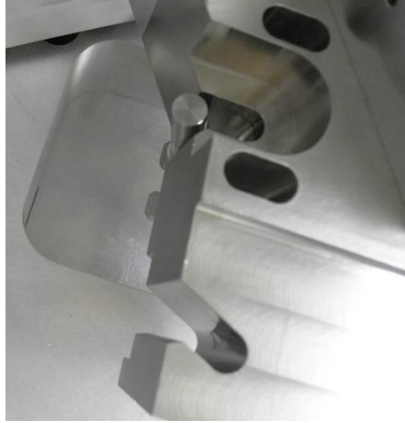
Figure 98: Top of Alignment Rod on D0902276 Stage 1 Flexure Rod Bracket (looking down from the top)
