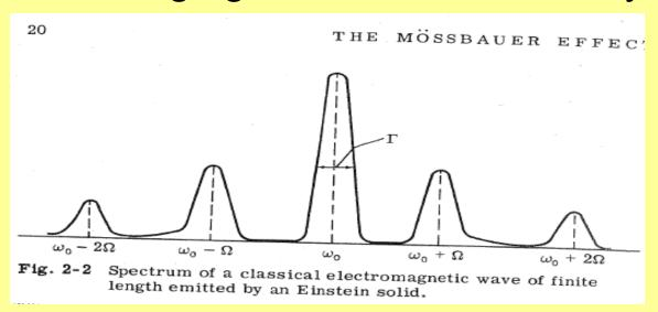
Lattice vibrations modulate the energy of  $\gamma$ -ray (Shapiro1960). Central unshifted line (ME line) emitted with natural width  $\Gamma$  Sidebands  $E_o \pm n\Omega$  (also with  $\Gamma$ );  $\Omega$  are the phonon frequencies. Condition for ME:  $\rightarrow \Gamma << \Omega$  i.e. lifetime of emitting level longer than typical lattice vibrational time  $1/\Omega \sim 10^{-14}$  sec
