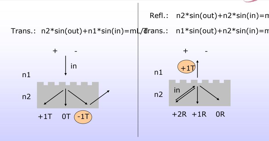
Between coupling in and out the sign of the diffraction order switches
