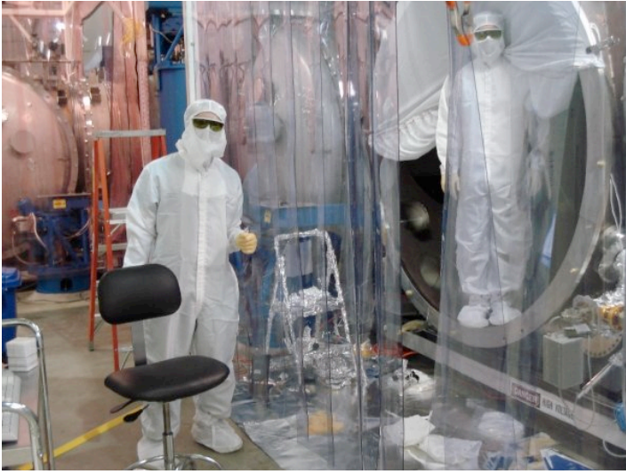
Figure 11: LIGO technicians work on internal optical components. Clean room protocols are used any time these components are exposed to atmosphere to prevent future vacuum contamination. [Image: D. Hoak]
