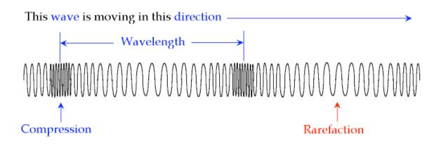
Now calculate the speed of a *longitudinal* wave in the Slinky. Gather several (about 5 or so) rings of the Slinky together. When you let go, you will see the compression travel the length of the Slinky. Time how long it takes the compression to travel the whole length (you will here the compression 'clink' against the attachment disk when it arrives at the end):
