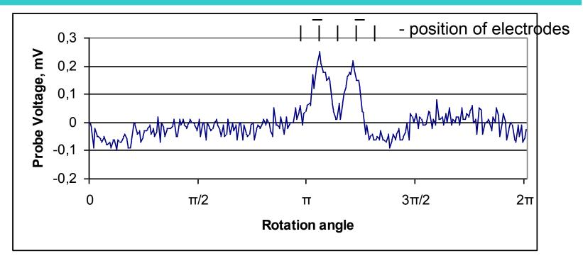
Polarization voltage of 600 V was applied to electrodes during 4 hours (Rough estimate of polarization charge density  $\sim 3 \times 10^9 \text{ e/cm}^2$ ) After switching off electric field:
