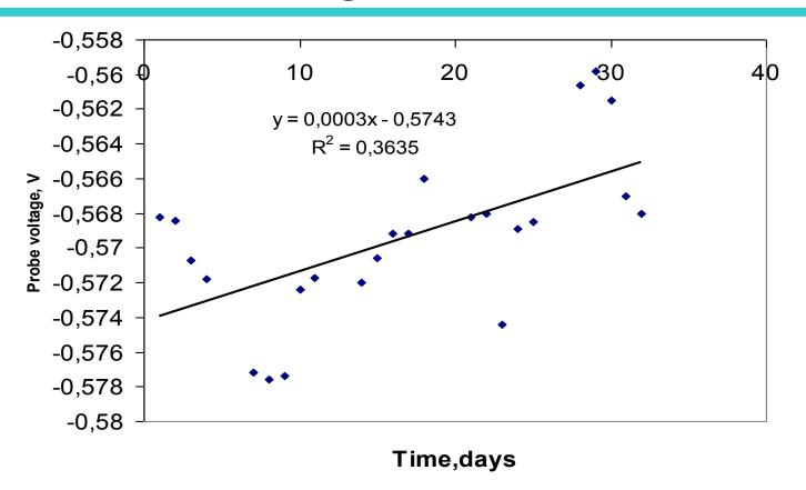
Time dependence of the negative charge peak amplitude for sample cleaned with FC&CNT (Decay time > 3 years)
