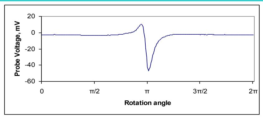
Amplitude of remanent polarization charge  $\approx 3 \times 10^7$  e/cm<sup>2</sup> (increase by a factor of **300** as compared with surface without scratch) Decay time of remanent polarization charge  $\approx 3$  hours (non-exponential law)
