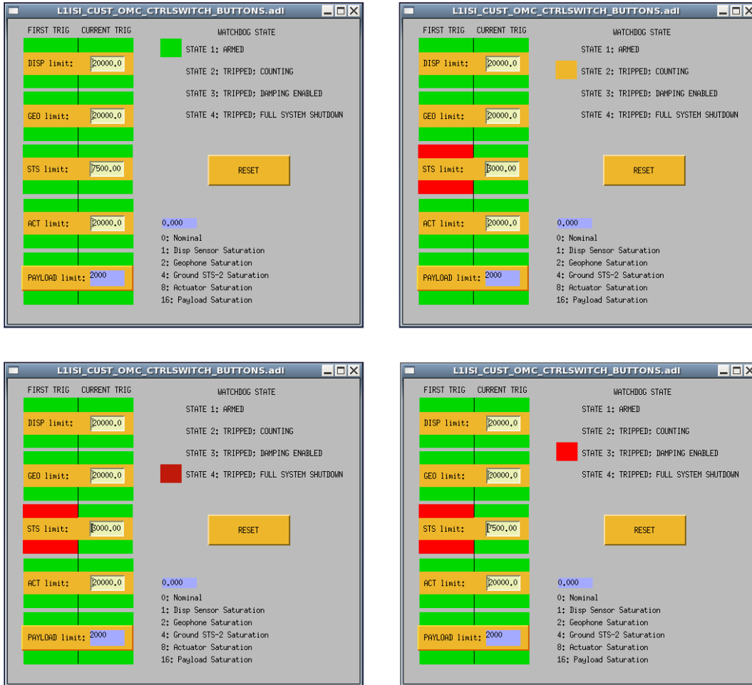
Figure 13: HAM ISI Watchdog MEDM screen. The four panels, starting in the bottom left and continuing clockwise (as in figure 1) show the screen in state 1, 2, 3, and 4.
