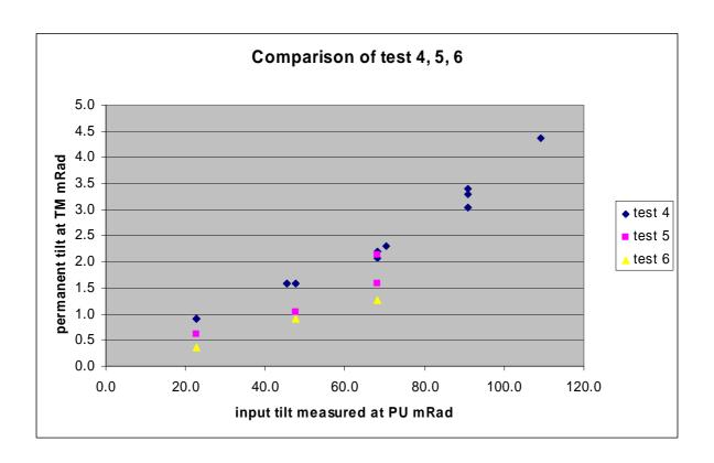
The effect is of the order of 0.02 mRad output per mRad input. An interesting observation is that, if this effect is linear down to small levels, an output tilt of 100 microRad would be produced by an input tilt of 5 mRad.
