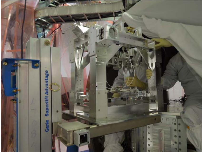
Figure 5. The OMCS on the Genie lift just before moving into HAM6. Note: the vibration absorbers should not be installed at this point.
