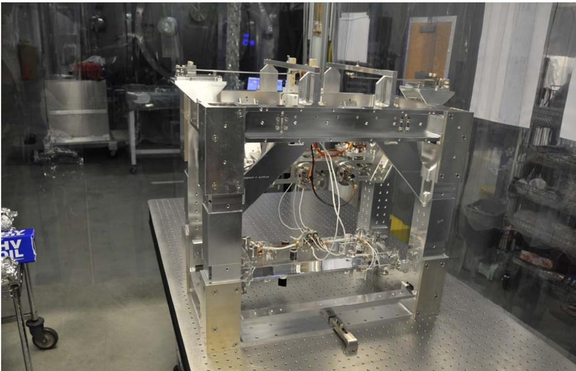
Figure 1. OMCS with OMC fused silica optics bench installed.
